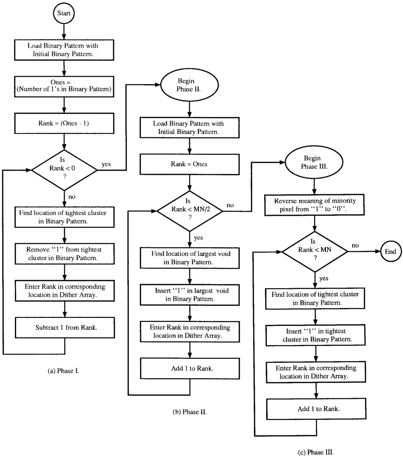
Figure 5: Dither Array Generator. (a) Phase I: Elements form  $(Ones-1)$  to 0 are entered. (b) Phase II: Elements form  $Ones$  to  $(\frac{MN}{2} - 1)$  are entered. (c) Phase III: Elements from  $(\frac{MN}{2})$  to  $MN$  are entered.
