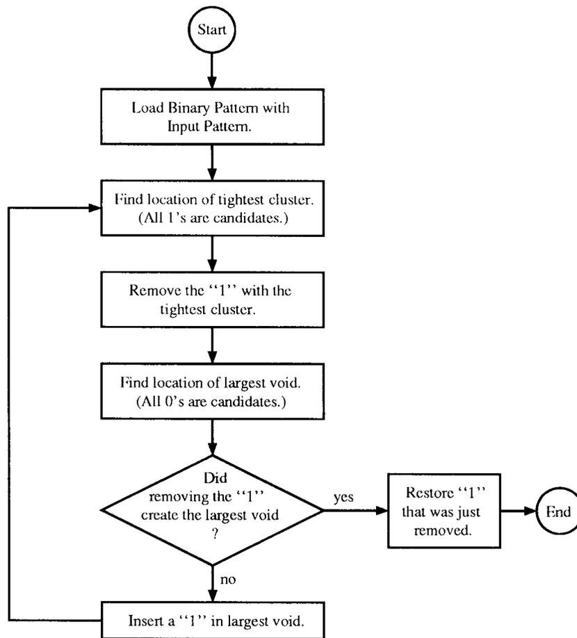
Figure 2: Initial Binary Pattern Generator.
