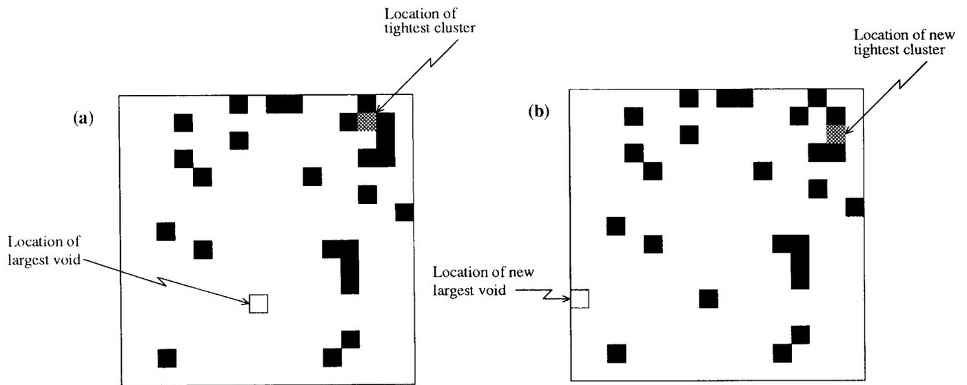
Figure 3: Example of the first two iterations of the Initial Binary Pattern Generator. The 16x16 Input pattern in (a) has 26 minority pixels (1's).
