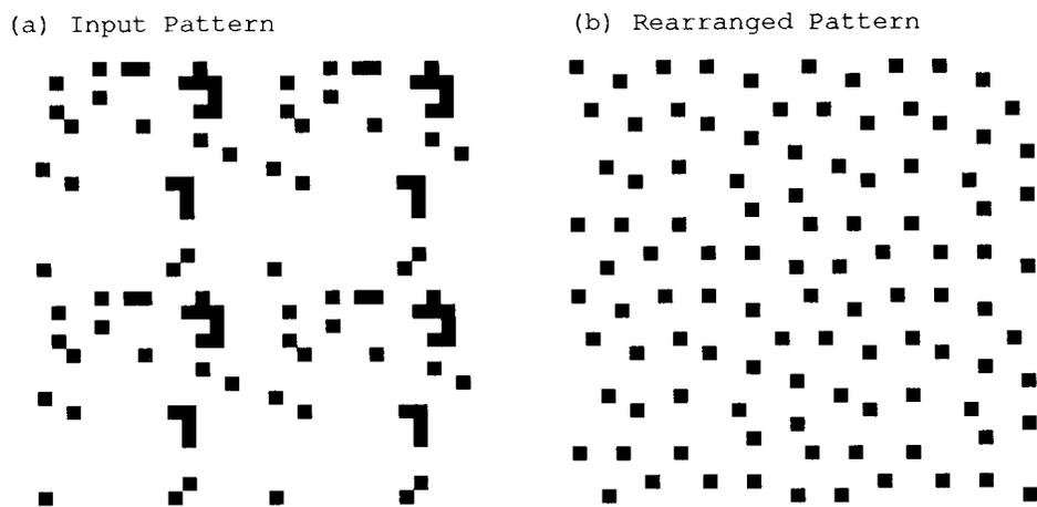
Figure 4: Results of the Initial Binary Pattern Generator. Four periods of the 16x16 Input pattern (a) and the Rearranged pattern (b) are shown to illustrate the wrap-around properties. The Input pattern is the same as that shown in figure 3(a).
